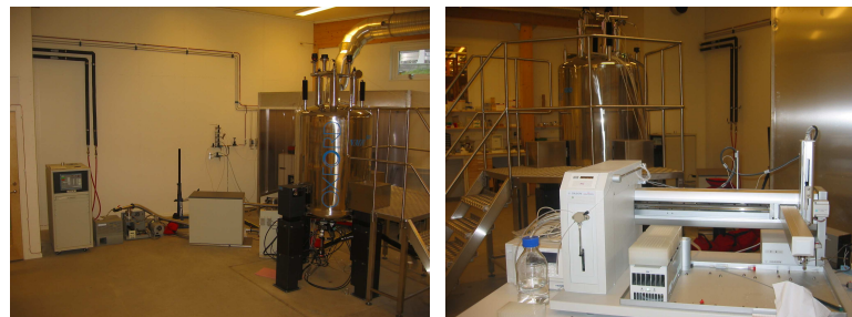
600 MHz Varian Unity NMR Spectrometer equipped with cold probe, Gilson robot with Peltier cooling element, flow cell
